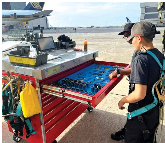
Pilot deployment of machine-vision-enabled smart tool chests.
