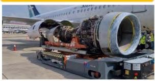
Collaboration with equipment manufacturer to develop an automated solution for engine change process
