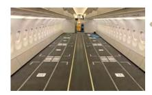
Solutions for passenger-to-cargo space conversion to increase cargo capacity of passenger aircraft
